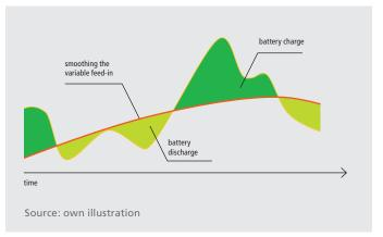
Battery storage can also be used to flatten the variable feedin of renewable energies such as wind and solar. This means that rapid power changes causing unwanted voltage and power fluctuations can be reduced or eliminated. For producers and traders, this means a reduction of the uncertainties in generation forecasts. As a result, balance group managers can adjust their balance groups more accurately and reduce inequality and the associated costs.
